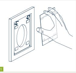
Hold the cover firmly on the right and left side. With your index and middle fingers, guide the top vent cover tabs to the top slots and insert them. Hold the cover at a slight angle.
