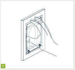
Insert the two flexible tabs into the free slots.
