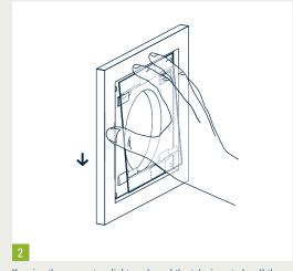
Keeping the cover at a slight angle and the tabs inserted, pull the cover toward the other two flexible tabs.
