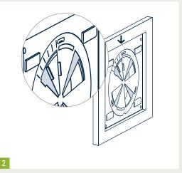
The volume flow regulator is infinitely variable. The markings on the edge of the volume flow regulator are orientation for setting the air current. They indicate the flow rate from 0 to 100 percent in increments of 20.
