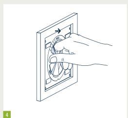
To remove the volume flow regulator, put your finger through the opened volume flow regulator and reach behind it. If there is a filter in it, reach carefully between the volume flow regulator and the filter. Press your thumb against the vent. Use the pressure of your thumb to carefully release the volume flow regulator from the connecting piece. The volume flow regulator is reusable. The filter can be exchanged with a replacement filter.
