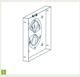
To remove the volume flow regulator, rotate the accessory in the vent by approx. 45 degrees to the left or right. With this you separate the notch and the anti-rotation device. Now the volume flow regulator can be easily removed. The volume flow regulator is reusable. The filter can be replaced by a replacement filter.
