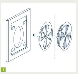
Insert the volume flow regulator - with the filter as required - frontally into the free connecting piece of the vent (e.g. Vent THREE) until it fits into place.
