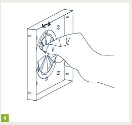
To regulate the supply and exhaust air, turn the volume flow regulator setting ring as required. If the volume flow regulator is combined with a filter, the exhaust air can be regulated and filtered at the same time. Now the cover can be installed (see instructions).
