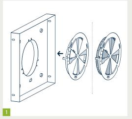
Insert the volume flow regulator - with the filter as required frontally into the free connecting piece of the vent. The accessory can be inserted in any position in the vent.
