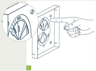
The volume flow regulator is infinitely variable. The markings on the edge of the volume flow regulator are orientation for setting the air current. They indicate the flow rate from 0 to 100 percent in increments of 20.
