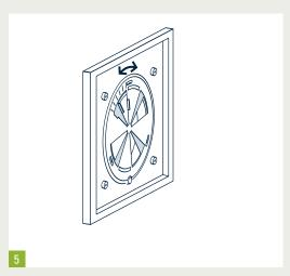
To remove the volume flow regulator, rotate the volume flow regulator in the vent by approx. 45 degrees to the left or right. This removes the notch at the accessory from the anti-rotation device. After that, the volume flow regulator can be easily removed. The volume flow regulator is reusable. The filter can be replaced by a replacement filter.
