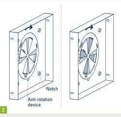
To fix the accessory, the notch on the volume flow regulator must be rotated to the anti-rotation device on the vent. The accessory is now firmly integrated into the vent.
