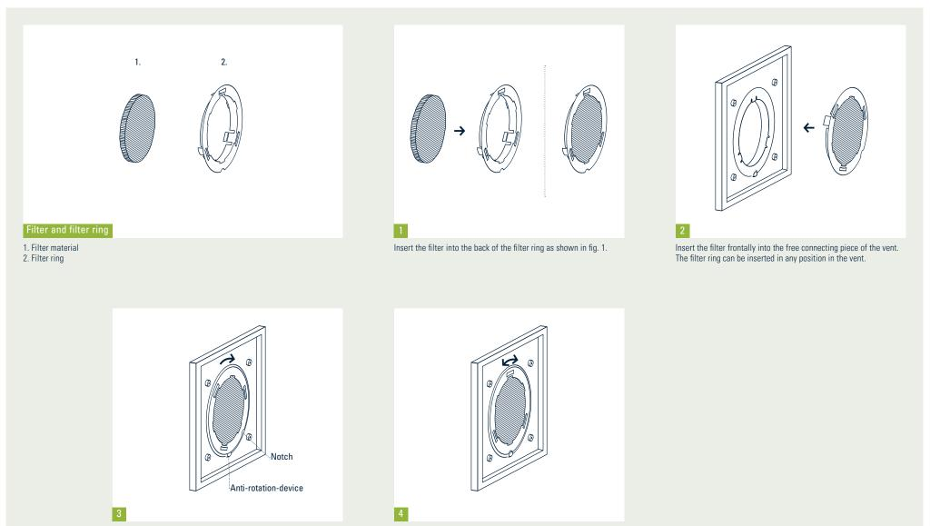
To fix the accessory, the notch on the filter ring must be rotated to the anti-rotation device on the vent. The accessory is now firmly integrated into the vent. The cover can be installed (see instructions).
