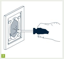
To replace the filter, insert a screwdriver or similar object into the slit between the filter ring and the filter material. Then use the screwdriver to pull the filter out of the ring. CAUTION: This may damage the filter ring and material.
