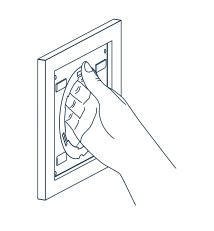
To disassemble the filter ring, put your hand through the ring and use the index finger to reach behind one of the three long filter prongs. Use your thumb and index finger to pull the prong out of the anchor. After removing all three prongs, pull the ring out of the vent connecting piece. The filter ring is reusable with a replacement filter.
