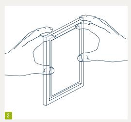
To disassemble the cover: Use both index fingers to reach behind two corners of the valve cover and press gently against the valve frame with your thumb.
