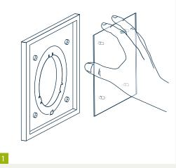
Insert all four retention bolts into the four bolt holders on the valve and gently press until the cover is flush to the valve frame.
